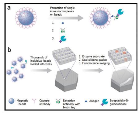
a. Single protein molecules are captured and labeled on beads.b. Beads are loaded into femtoliter-volume well arrays for isolation and detection of single molecules by fluorescence imaging.
